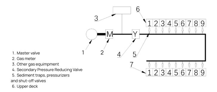
Gas-heated dryers need to arrange piping in advance, refer to Table 4, 5, 6 and Fig. 8 to calculate the size of piping.
